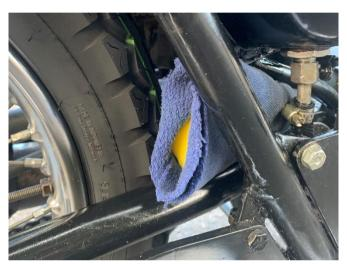
from the tool kit rag supply, could be jammed between the bottom of the rear mudguard and the swinging arm pivot, the aim being to soak up some excess oil and/or divert it away from the rear wheel. A can of degreaser later (thanks Bill) and a wipe of the tyre, and we were away on our final jaunt back to Ulverstone.
